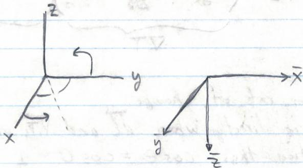
$$\begin{aligned}\bar{A}_x &= A_y \\ \bar{A}_y &= A_x \\ \bar{A}_z &= -A_z\end{aligned}$$
