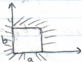
$$-\frac{m^2 \pi^2}{a^2} - \frac{n^2 \pi^2}{b^2} + \left( \frac{\omega}{c} \right)^2 - k^2 = 0 \Rightarrow k = \sqrt{\frac{\omega^2}{c^2} - \frac{m^2 \pi^2}{a^2} - \frac{n^2 \pi^2}{b^2}}$$
