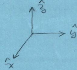
$$\begin{aligned} d\vec{F} &= I d\vec{l} \times \vec{B} \\ &= I d\vec{l} \times \frac{\mu_0 I}{2\pi s} \hat{x} \\ &= I d\vec{z} \times \frac{\mu_0 I}{2\pi s} \hat{x} \\ &= \frac{\mu_0 I^2 d\vec{z}}{2\pi s} \hat{y} \end{aligned}$$
