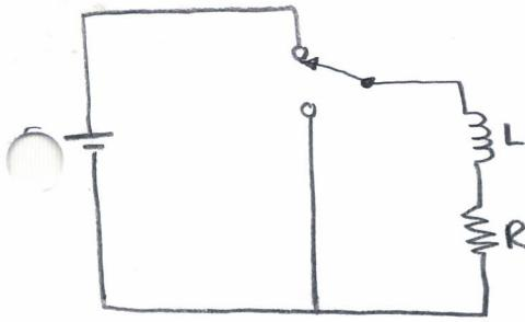
Suppose this circuit has been connected as shown when at  $t=0$  the battery is disconnected and the  $L/R$  combination is left to drain.
