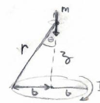
$$\checkmark \Phi = \oint \vec{A} \cdot d\vec{l} = \frac{\mu_0 a^2 \pi I}{4\pi} \oint \frac{\sin \theta}{r^2} \hat{\phi} \cdot b d\hat{\phi} \quad \sin \theta = \frac{b}{r} : r = (z^2 + b^2)^{1/2}$$
