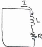
$$L \frac{dI}{dt} + IR = 0 \Rightarrow \frac{dI}{I} = -dt \left( \frac{R}{L} \right) \Rightarrow \ln I = -t \left( \frac{R}{L} \right) + \text{const.}$$
