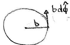
$$\vec{B} = \frac{\mu_0 I}{4\pi(z^2 + b^2)} \oint \frac{-b^2 \hat{z}}{(z^2 + b^2)^{3/2}} = \frac{-\mu_0 b^2 I \hat{z}}{2(z^2 + b^2)^{3/2}} = \vec{B} \text{ (at center of loop of radius } a)$$
