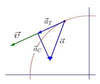
Here  $\vec{a}_c = -\frac{v^2}{R}\hat{r}$  whereas  $\vec{a}_T = \frac{dv}{dt}T$ . We can have  $\vec{a}_T = 0$  however the same is not true for the centripetal part. If the motion is circular then there has to be a center-seeking component of the acceleration with magnitude given by  $v^2/R$ .
