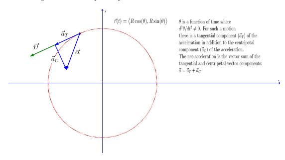
Notice the magnitude of the acceleration in the above example is given by  $a = \sqrt{R^2\omega^4 + R^2\alpha^2}$ . If  $\alpha = 0$  then the formula reduces to  $a = R\omega^2$  in good agreement with the previous example.
