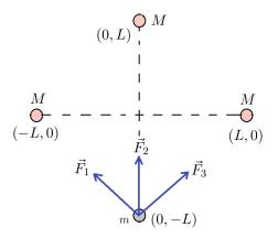
**Solution:** Let us set-up the forces of gravity for each mass pictured above:
