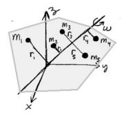
Pictured above is a solid object and some representative bits of mass inside the object. Each little bit of mass dm is located at distance r from the axis pictured. Notice that the speed of dm is thus given by  $v = r\omega$  since the motion in question involves no radial motion. The kinetic energy of the dm is given by
