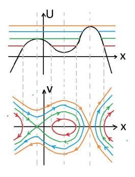
**Example 5.5.1.** The Poincare plot for the spring without friction is as follows:
