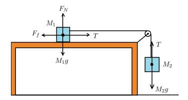
**Example Problem 4.1.6.** Consider mass  $M_1$  and  $M_2$  connected by a rope of very small mass over a pulley with neglible mass. Let  $\mu_k$  be the coefficient of kinetic friction between the inclined plane pictured below and the masses which are put in motion to the right. Find the acceleration of the system taking rightward overall motion as positive.
