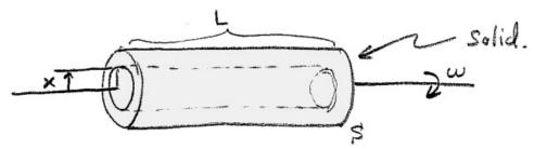
To find the mass dm of such a slice we solve the density  $\rho = \frac{M}{\pi R^2 L} = \frac{dm}{dV}$  to see  $dm = \frac{M}{\pi R^2 L} dV$ . But, notice  $dV = (2\pi x L) dx$  if we imagine cutting the the cylindrical shell of thickness dx lengthwise and laying it flat with length L and width  $2\pi x$ . The moment of inertia dI from our shell is given by  $dI = x^2 dm$  which gives:
