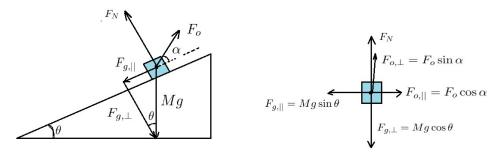
The free body diagram has gravity pictured as two components. Notice the acceleration is nontrivial only in the parallel direction. We expect  $a_{\perp} = 0$  since the box is on the plane. Notice:
