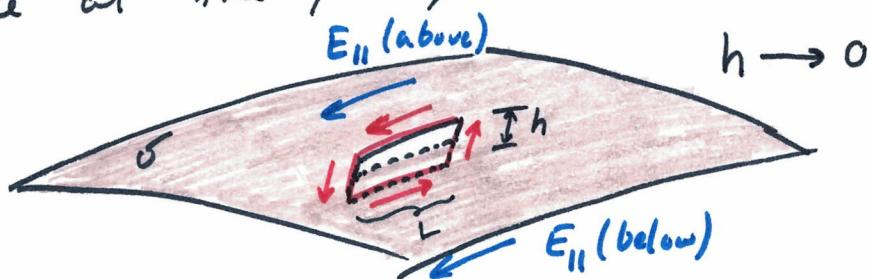
$$\oint_C \vec{E} \cdot d\vec{l} = 0 = E_{\parallel}(\text{above})L - E_{\parallel}(\text{below})L$$
