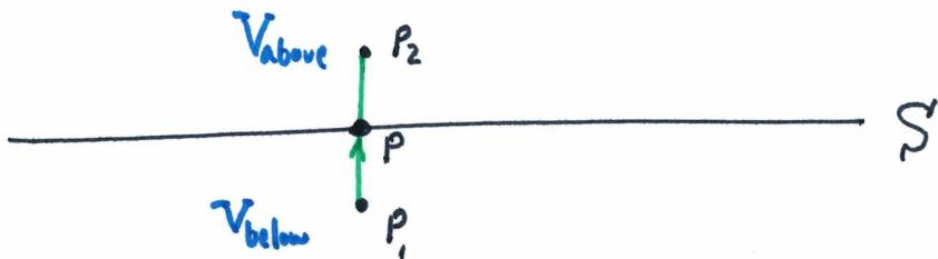
$$V_{\text{above}} - V_{\text{below}} = - \int_{P_1}^{P_2} \vec{E} \cdot d\vec{l} \rightarrow 0 \quad \text{as } P_1, P_2 \rightarrow P.$$
