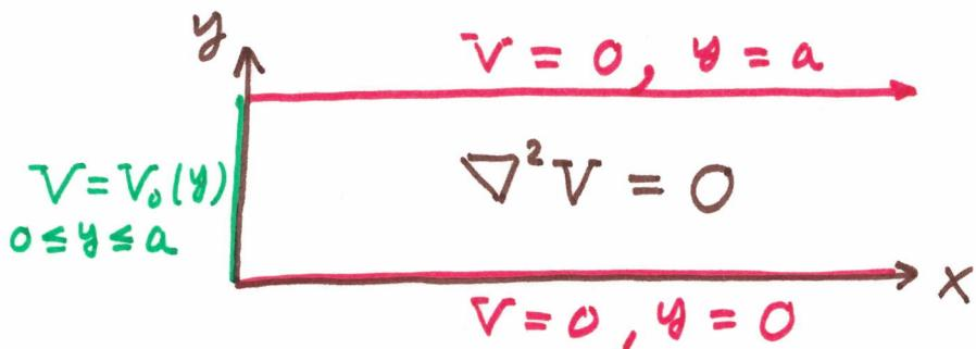
$$\frac{\partial^2 V}{\partial x^2} + \frac{\partial^2 V}{\partial y^2} + \frac{\partial^2 V}{\partial z^2} = 0$$
