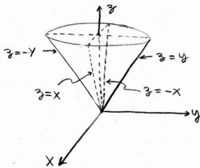
the trick is to draw the shape you imagine then check it with the cross-section lines (the text calls these "traces")
