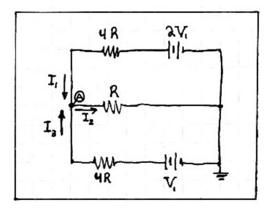
Conservation of charge implies the sum of currents into a node must equal the sum of the currents flowing out of the node. We use Ohm's  $Law\ V = IR$  to set-up the currents, here V should be the voltage dropped across the resistor R.
