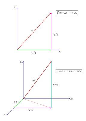
Notice these pictures go to show how you can break-down vectors into component vectors which point in the direction of the coordinate axis. Vectors of length<sup>2</sup> one which point in the coordinate
