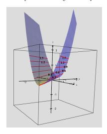
**Example 7.9.13.** Consider the quadric form Q(x,y) = 4xy. It's not immediately obvious (to me) what the level curves Q(x,y) = k look like. We'll make use of the preceding proposition to understand those graphs. Notice  $Q(x,y) = [x,y] \begin{bmatrix} 0 & 2 \\ 0 & 2 \end{bmatrix} \begin{bmatrix} x \\ y \end{bmatrix}$ . Denote the matrix of the form by A and calculate the e-values/vectors:
