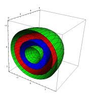
Finally, let's take a moment to write  $Q(x,y,z) = [x,y,z] \begin{bmatrix} 1 & 0 & 0 \\ 0 & 2 & 0 \\ 0 & 0 & 3 \end{bmatrix} \begin{bmatrix} x \\ y \end{bmatrix}$  in this case the matrix is diagonal and we note that the e-values are  $\lambda_1 = 1$  and  $\lambda_2 = 2$  and  $\lambda_3 = 3$ .
