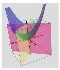
**Example 7.9.12.** Consider the quadric form  $Q(x,y) = x^2 + 2xy + y^2$ . It's not immediately obvious (to me) what the level curves Q(x,y) = k look like. We'll make use of the preceding proposition to understand those graphs. Notice  $Q(x,y) = [x,y] \begin{bmatrix} 1 & 1 \\ 1 & 1 \end{bmatrix} \begin{bmatrix} x \\ y \end{bmatrix}$ . Denote the matrix of the form by A and calculate the e-values/vectors:
