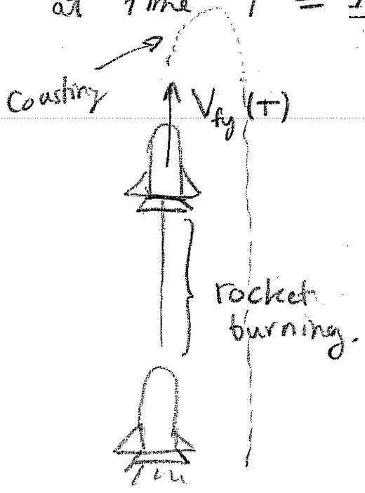
for  $t \geq T$  it's a free-fall problem with  $M = M_{\text{ROCKET UNFUELED}}$ .
