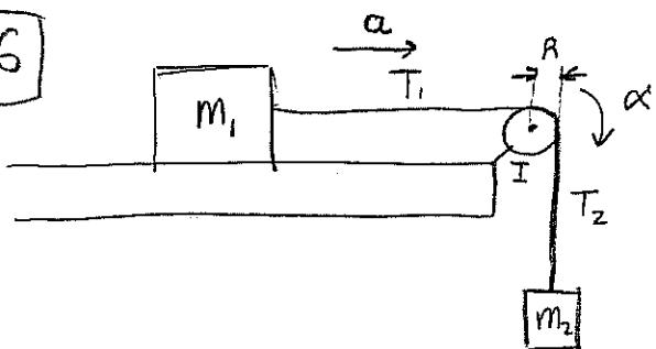
Suppose the blocks pictured are connected by a massive pulley with moment of inertia  $I$  and radius  $R$ . If the table is frictionless and the rope does not slip find  $a$  and  $\alpha$
