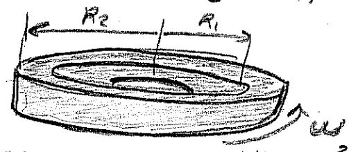
A flywheel serves as a type of battery. It stores energy as KE whereas others use chemical, electrical or even gravitational energy. The idea of using a flywheel to power an electric car has been around for decades. Apparently no profitable design exists.
