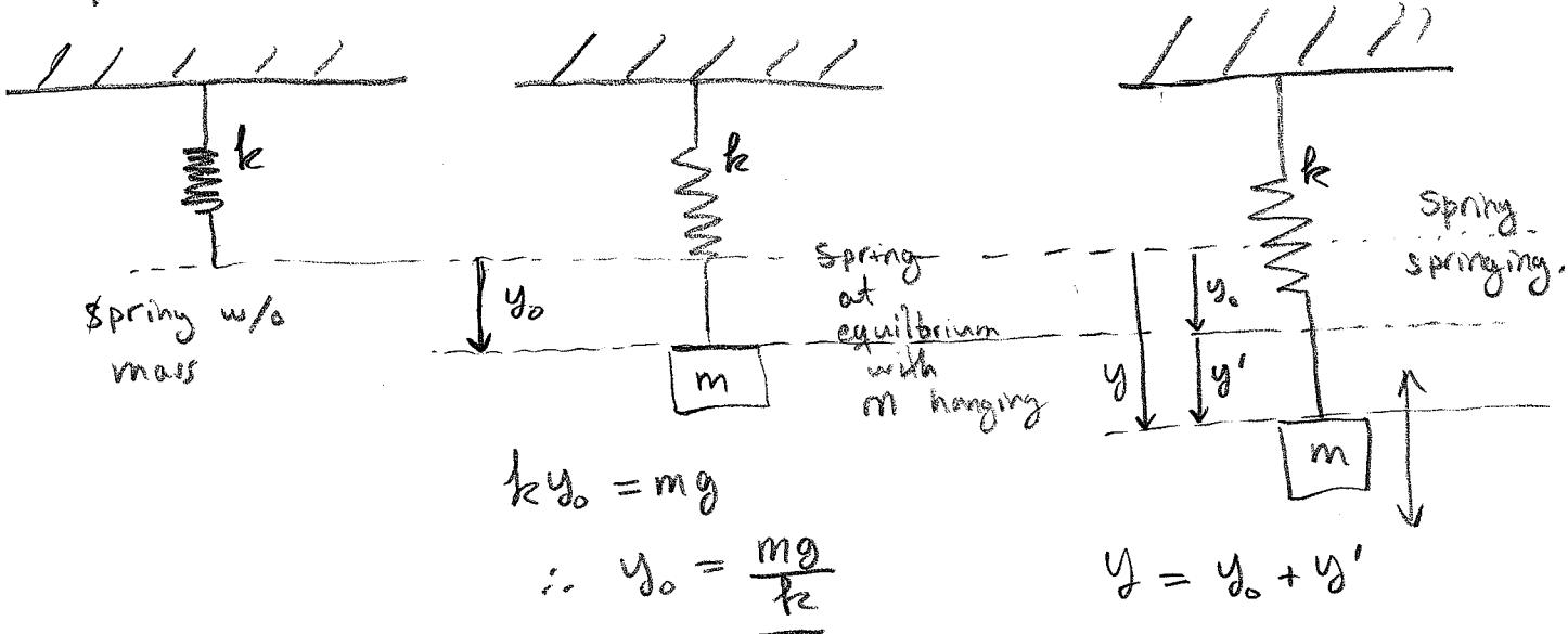
Forces on m:  $-ky + mg = F_{\text{net}}$  (down is positive)
