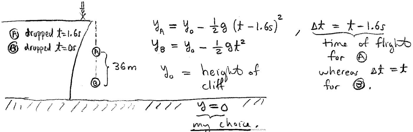
$$\begin{aligned} \text{Given } y_A - y_B &= 36 \text{ m} = \frac{1}{2}g(t-1.6s)^2 + \frac{1}{2}gt^2 \\ \Rightarrow \frac{72 \text{ m}}{g} &= t^2 - [t^2 - (3.2s)t + 2.56s^2] \\ \Rightarrow t &= \frac{72 \text{ m}/g - 2.56s^2}{3.2s} \approx 1.4936s \\ \Rightarrow |y_A - y_0| &= \frac{1}{2}gt^2 = \frac{(9.81 \frac{\text{m}}{\text{s}^2})(1.4936s)^2}{2} = 10.94 \text{ m} \end{aligned}$$
