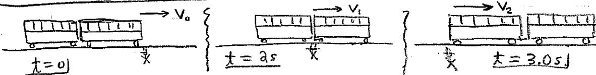
$$V_{\text{avg}(1)} = \frac{10 \text{ m}}{2 \text{ s}} = 5 \frac{\text{m}}{\text{s}} = \frac{1}{2}(V_0 + V_1) \Rightarrow V_0 + V_1 = 10 \frac{\text{m}}{\text{s}}$$
