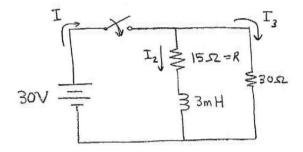
**Problem 39** Find the currents and voltages indicated below (assume the circuit has been connected a long time)
